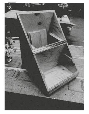
The production of these custom handles to a right size (most industrial handles were not solid enough, too small, too big, too round, etc) turned out to be a very specific and difficult process. The wheels needed to support the heavy load were expensive, and it remains hard to pilot on uneven grounds.
