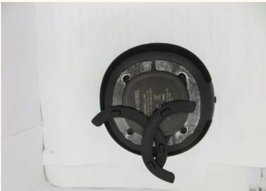
fig 6. This speaker had no visible screws on the outside. 4 screws where found removing glued on protective caps
