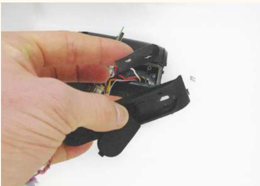
fig 7. The last screw was even better hidden. It was found behind a sticker labeling the two input ports of the device
