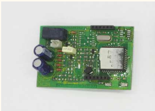
fig 8. Manufacturer deliberately obscured the label of this chip
