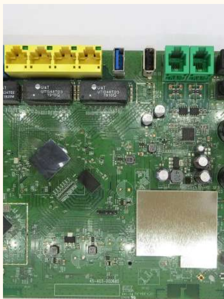
fig 16. Smaller components are difficult to desolder
