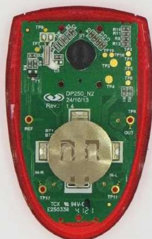
fig 17. The blob cannot be removed
