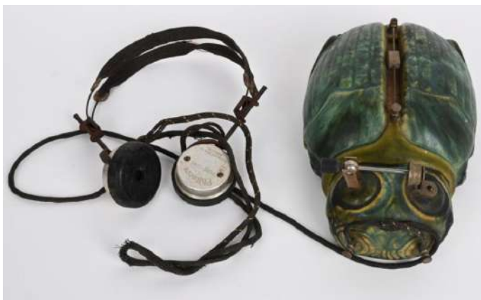
Figure 3. The Mystic Bug crystal radio manufactured by Brush-McCoy in 1926.
